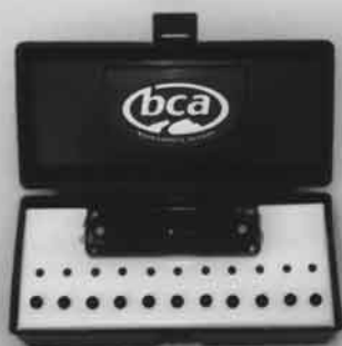
Control panel for an 11 transmitter system--Summit Huts will install a one 6 and one 4 transmitter system at Francie's and Jane's. A toggle switch controls how many transmitters are "on" (transmitting) at any time, thereby controlling how difficult a scenario the user is working on.
